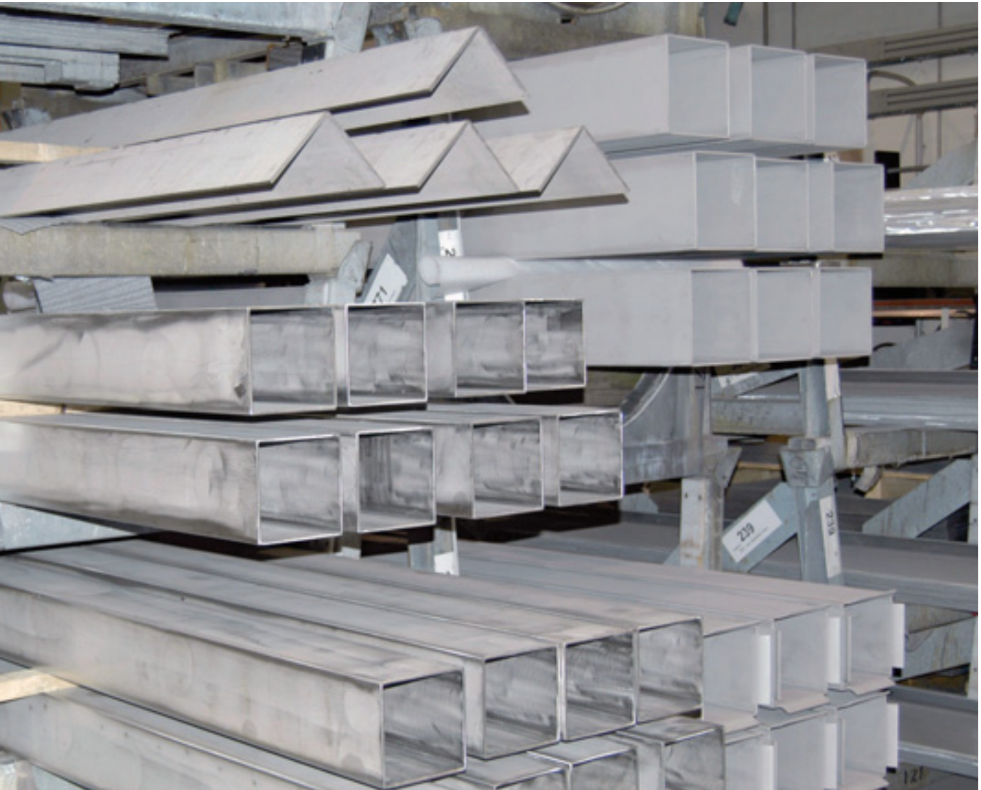
State-of-the-art welding technology: Rectangular ducts welded by laser technology for wet storage
