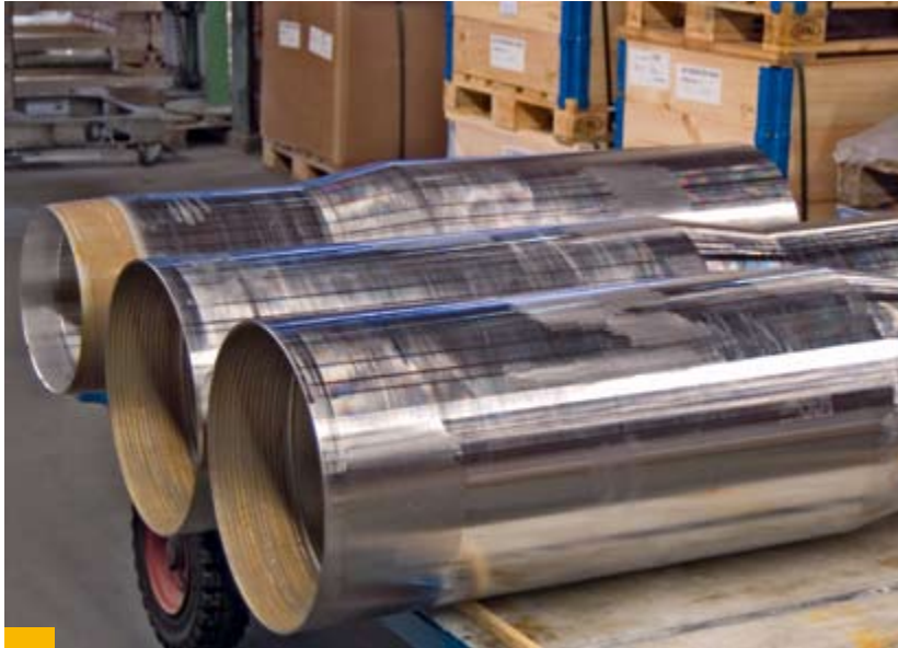
The initial product for our components is the high-quality pipe we ourselves produce: cross over subs 13 3/8" / 16" in Alloy 625
