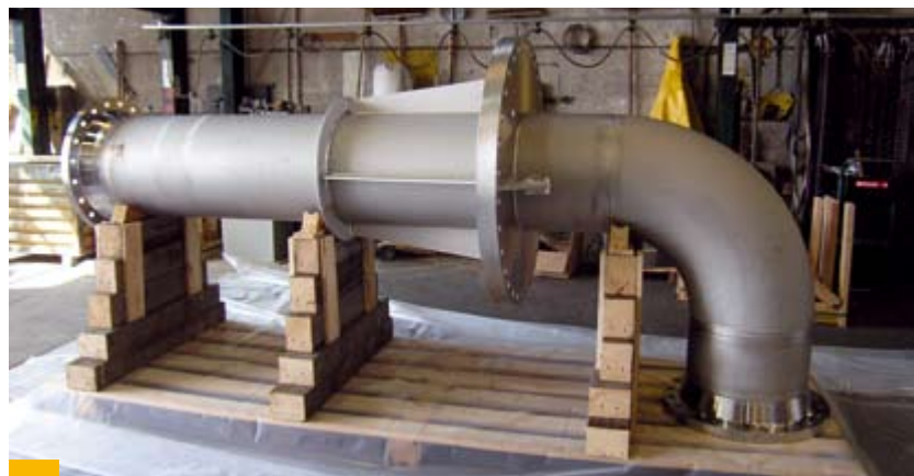
Ready-to-install spools – prefabrication in our plant ensures good quality
